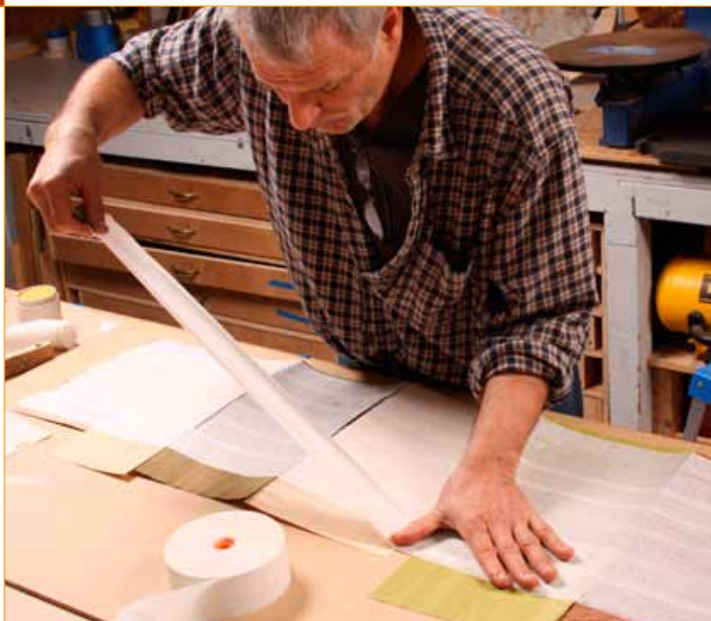
Reinforce the veneers first. Put veneer tape on the “show” faces. Wet the tape on a damp sponge, and burnish it afterward with a brass-bristle brush to improve its bond. Place the sheets under MDF to keep them flat while drying.
