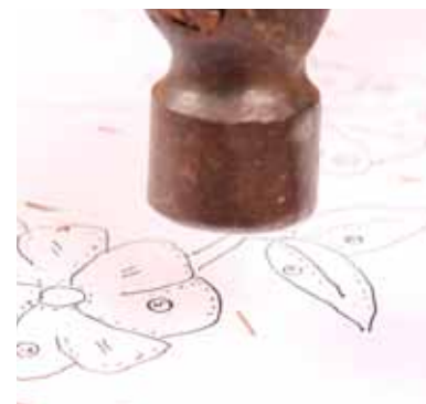
Clinch the pins. Bend over each pin in the same direction above and below for greatest strength and to avoid shifting the layers.
