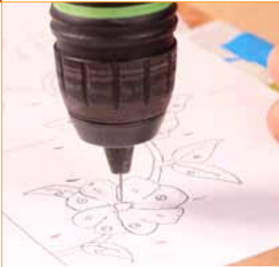
Starter hole. Schürch cuts the head off an 18-gauge nail and chucks it in a drill to create a starter hole for the scrollsaw. The nail parts the wood fibers, leaving an undetectable hole.
