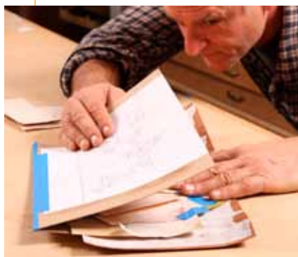
The flip trick. To see where each piece of veneer should go, flip the top of the packet up and down quickly. Secure each piece with a few strips of blue tape.
