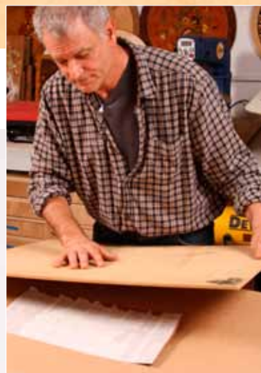
One last layer to remove, then let it dry. Don't forget the blue tape you put on the glue face (above)! Put the veneer under a layer of MDF to keep it flat while it dries (right).
