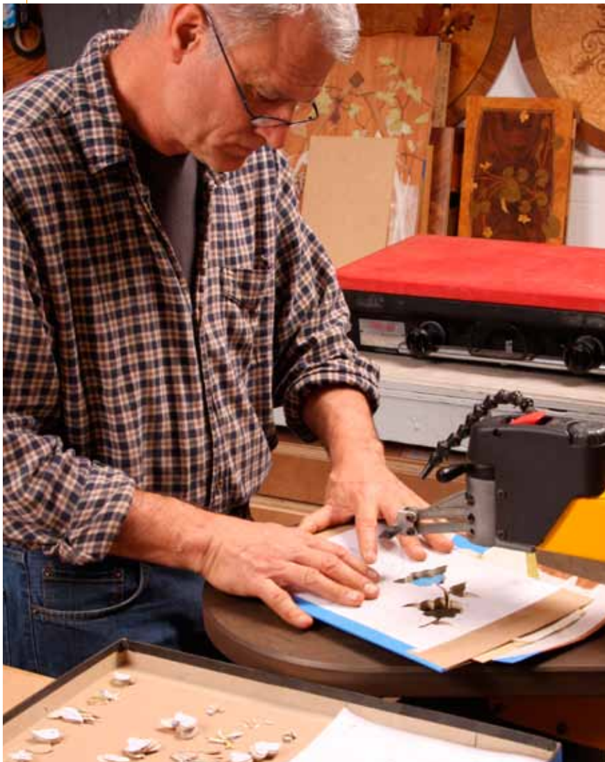
Stay organized. Under each part of the drawing is a small stack of veneer parts. Keep each stack together, with its labeled piece on top. Use a big tray and another copy of the drawing to keep track of the pieces.
