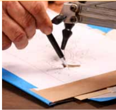
One stack at a time. After sawing an element free, press down on it with a pencil, lift the packet, and then reach under it to remove the small stack of pieces.
